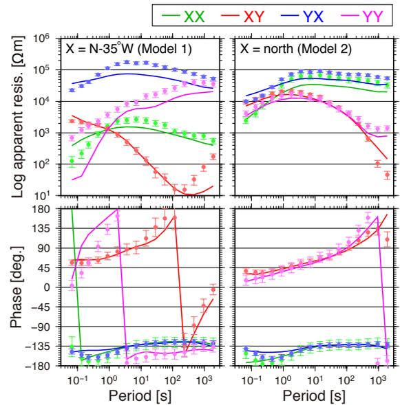
**Figure 3.** Observed (dots) and calculated (lines) sounding curves at the site D04 in the two rotation azimuths. See figure 4 for the explanations of model 1 and 2.
