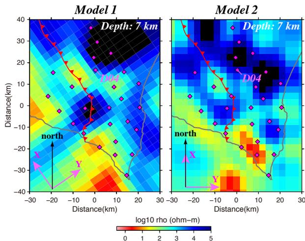
**Figure 4.** Horizontal resistivity distribution of the model 1 and 2 at depth 7.0 km. The x-axes of impedance tensor were settled to 0 and 325 degrees for model 1 and 2, respectively. Other inversion conditions were same for the both models (periods: 16 periods between 0.00667 and 1800 seconds, time steps: 5). Diamonds denote MT sites. The grey and red lines denote coastline, Hidaka Main Thrust, respectively. The RMS misfits are 1.07 and 1.27 for the model 1 and 2, respectively.
