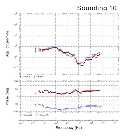
**Figure 5.** The apparent resistivity and phase recorded at site no. 10 for both TE and TM modes.
