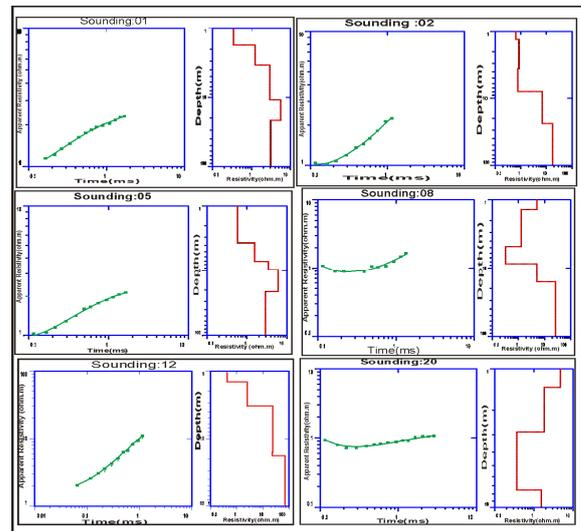
Figure 4. Examples of interpreted models for TEM curves measured in this study
