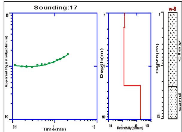
Figure 3. Calibration of the TEM station17 with the lithology of well 8
