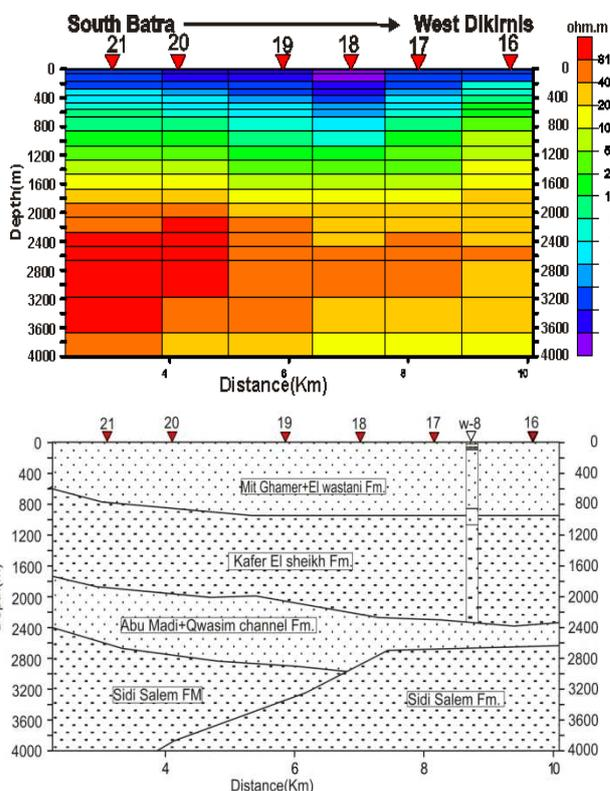
**Figure 6.** 2D inversion resistivity model along profile extended from South Battra to West Dikirmis and its geological cross section
