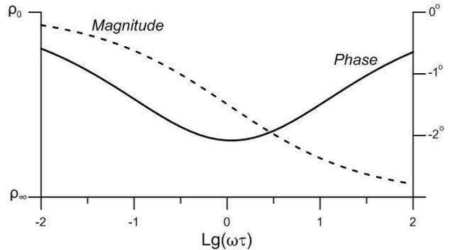
**Figure 1.** Amplitude and phase of Cole-Cole function.
