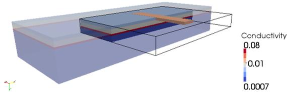
**Figure 2.** Sketch of the conductivity structure used for providing synthetic data.
