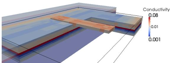
**Figure 4.** Conductivity distribution obtained after 12 Gauss-Newton steps.
