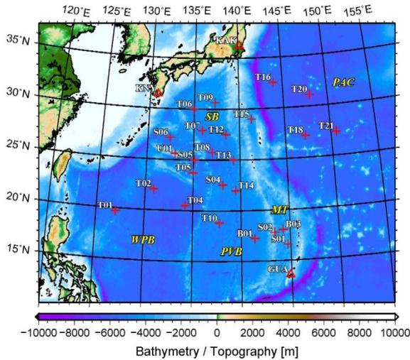
**Figure 1.** Location of the marine MT sites (red crosses) superimposed on a bathymetric map. Red triangles indicate the geomagnetic observations from which data were used as remote references for the response estimation. PAC, Pacific Plate; MT, Mariana Trough; SB, Shikoku Basin; PVB, Parece Vela Basin; WPB, West Philippine Basin.
