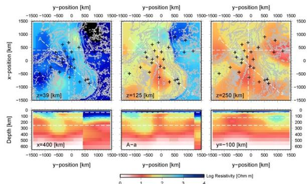
**Figure 3.** The best electrical conductivity model. The top panels show plane views at 39, 125 and 250 km depths, respectively. The bottom panels show cross-section views. Gray lines indicate bathymetric feature. Black crosses indicate MT sites. White dashed lines
