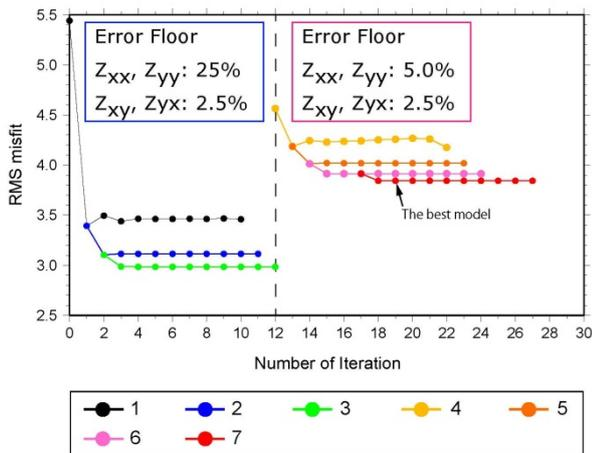
**Figure 2.** RMS misfit versus number of iteration for the inversion analysis. Color indicates an inversion step.
