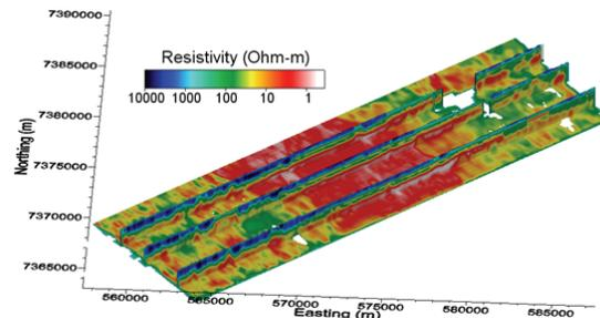
**Figure 2.** A perspective view of inverse 3D resistivity model.
