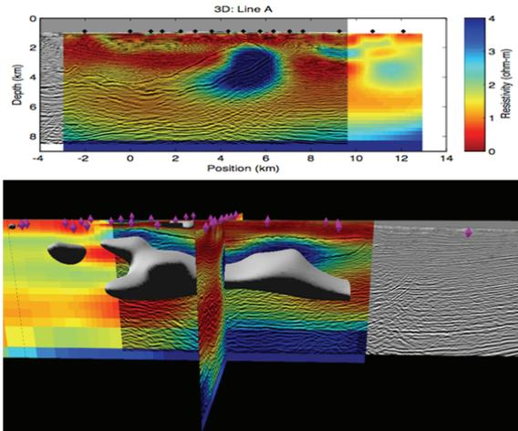
**Figure 1.** A vertical cross-section (top) and a 3D view (bottom) of the resistivity model overlapped with seismic sections.
