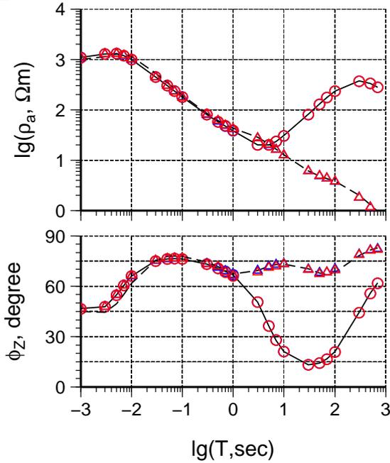
**Figure 3.** Accuracy of the forward solution. Comparison of the MT sounding curves over the center of the 2D prism. 2D forward responses computed from ModEM 2D: black solid line –  $Z_{yx}$ , dashed line –  $Z_{xy}$ . 3D responses computed from ModEM 3D original version: blue open circle –  $Z_{yx}$ , blue triangle –  $Z_{xy}$ . 3D responses computed from ModEM MG 3D with five coarseness levels: red open circle –  $Z_{yx}$ , red triangle –  $Z_{xy}$ .
