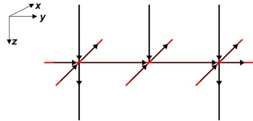
**Figure 2.** Discretization of the divergence on the interfaces. Red color represents interface layer from finer to coarser sub-grids.
