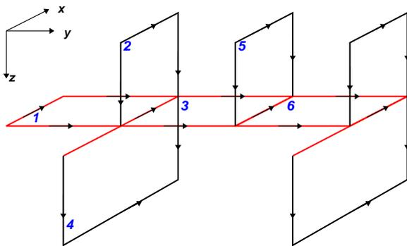
**Figure 1.** Discretization of the  $\mathbf{C}^\dagger \mathbf{C}$  operator on the interfaces. Red color represents interface layer from finer to coarser sub-grids.
